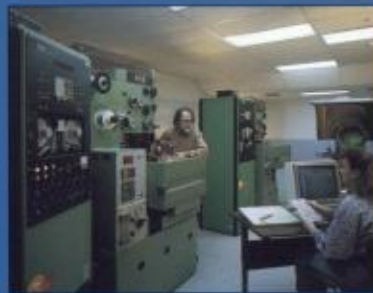
Precision cutting of CBN form tools and grooving tools. Design engineers operate our CMC wire EDM systems.
